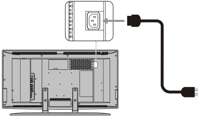
2. Connect the other end of the power cord to the wall outlet.
