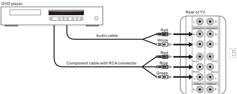
**Note:** The Y, Pb and Pr jacks do not provide audio, so audio cables must be connected to provide sound.
