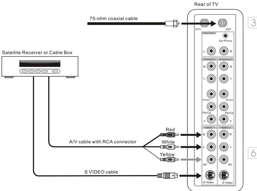
**Note:** When you connect video equipment to both the same Video and S Video input jacks, display will automatically select S Video first. To view S Video signal, please disconnect Video jack or turn off the Video signal on the video equipment.
