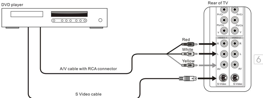
**Note:** When you connect video equipment to both the same Video and S-Video input jacks, the display will automatically select S-Video first. To view Video signal, please disconnect the S-Video jack or turn off the Video signal on the video equipment.
