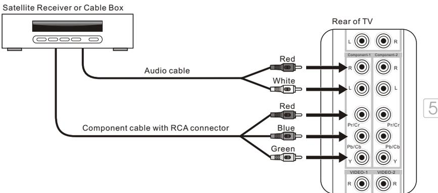
**Note:** The Y, Pb and Pr jacks do not provide audio, so audio cables must be connected to provide sound.
